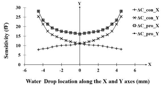
Figure 6: Sensitivity concerning water drop position along the X-axis and Y-axis in the CP plane.
