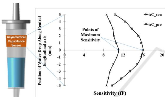
(b) Tapered cylindrical IV drip chamber with asymmetrical electrodes
