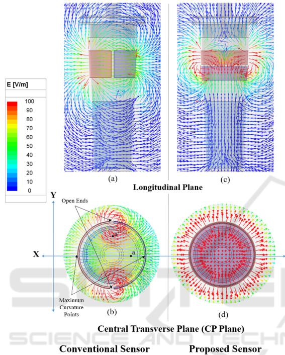
Figure 4: Electric field distribution in the longitudinal and CP plane of the asymmetrical capacitive sensors.
