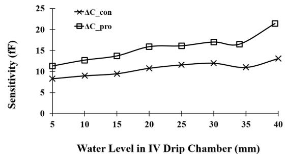
Figure 7: Sensitivity concerning water level within the IV drip chamber.
