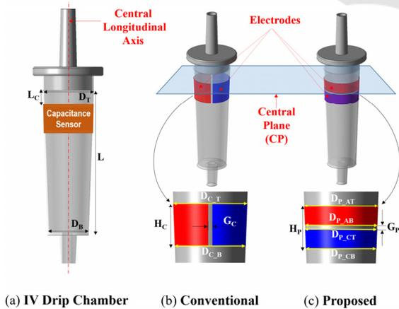
Figure 2: Standard IV drip chamber and capacitive sensors with asymmetrical electrodes.
