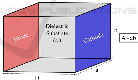
Figure 1: Simple parallel plate capacitor.
