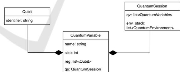
Figure 3: The Eclipse Qrisp Meta-Model for QuantumVariables - the key structure for qubit Management.
