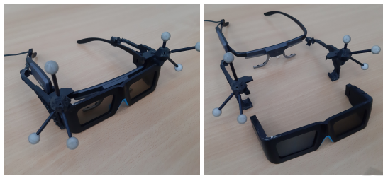
Figure 3: An assembly combining a system of Vulfoni stereoscopic glasses with Tobii 2 eye tracking glasses, attached together with a 3D-printed clip which is also designed as the tracking constellation system.
