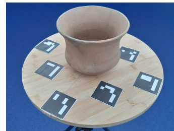
Figure 4: Augmented Reality markers (ArUco fiducial markers) placed around the object of interest in order to track the participants' position relative to the object.
