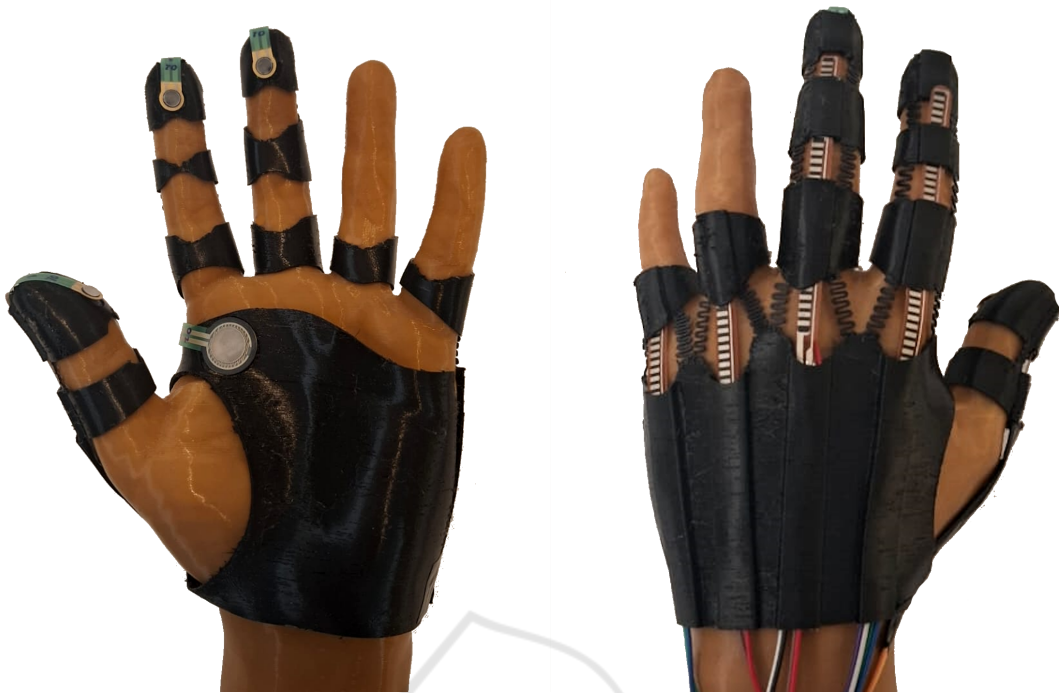
Figure 4: 3D Printed Orthosis with Sensors for Finger Movement and Grip Force Monitoring. Author.
