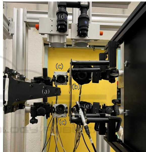
Figure 1: Photograph of the experimentation setup: (a) convergent nozzle, (b) slotted plate, (c) high-frequency cameras, (d) laser emitter, and (e) microphone.
