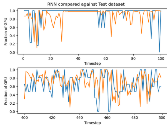
Figure 9: RNN tasked with reconstructing the test dataset. Orange is generated values and blue is true values. The X-axis is time. The Y-axis specifies what fraction of a GPU a task at a specific step requires with a max of 1 and 0 as minimum. It is evident from the figure that RNN can reconstruct data, although much worse than the other two models.
