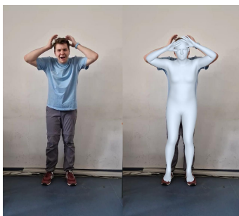
Figure 6: 3D mesh, extracted with ScoreHMR. Although the mesh was extracted in less time compared to SMPLify-X, it cannot reproduce the facial and hand expressions and still outputs the position of the hands incorrectly.
