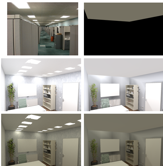
Figure 13: Output rendering and optimization. Top row: original image and target ceiling colour. Middle row: rendering of the initial state white light and arbitrary intensity. Bottom row: optimized light colour and intensity. The right column shows the corresponding simplified view used internally by the optimization framework.
