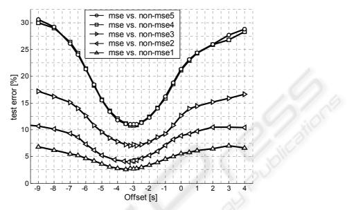
**Fig. 2.** Mean empirical test errors vs. segment offset parameter. OLVQ1 was utilized for classification of clear MSE vs. five different types of Non-MSE (see text). The length of signal segments was 8 sec.
