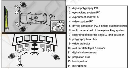
Fig. 1. Real car driving simulation laboratory
