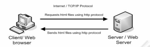
Figure 1: Simplified Client/Server of HTTP communication.
