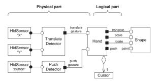
Figure 3: The "hand" instrument
