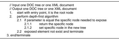
Figure 10: An algorithm for exposing specific node of Doc tree
