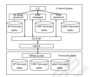
Figure 5: MPLS VPN software architecture.
