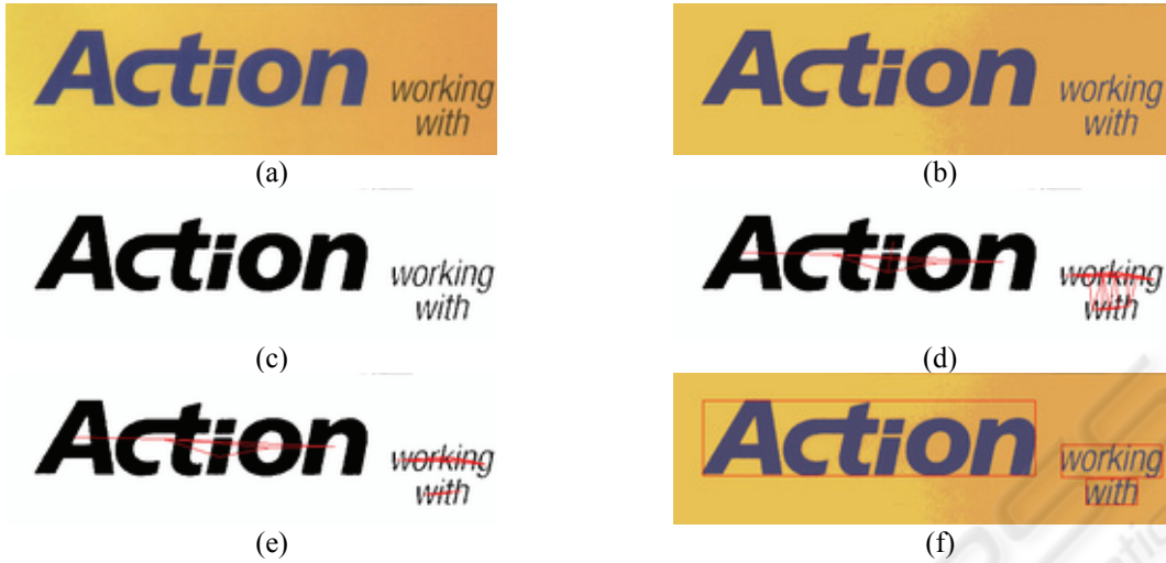
Figure 4: (a) Original color document, (b) After color reduction (4 colors), (c) Color plane 1, (d) initial grouping, (e) false connections removal, (f) final text localization after superimposition of all color planes.
