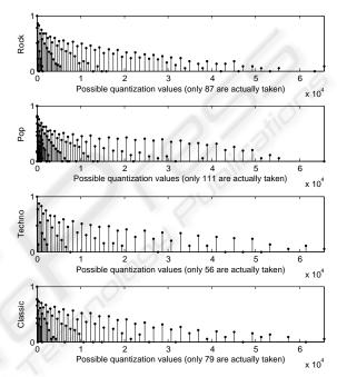
Figure 3: Histogram of the spectral quantization values for nearly transparent coding using FPQ for four 8-second musical excerpts named *Rock*, *Pop*, *Techno*, and *Classic*. according to their music style. Values are quantized using 16 bits (the dynamic range is therefore 0-65535). Vertical axis is in logarithmic scale and normalized to 1 for better visualization.
