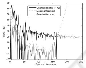
Figure 1: Short spectral frame of a music signal quantized using FPQ. Note that quantization error does not exceed the masking threshold at any point.
