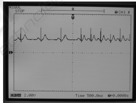
Figure 7: Simulated ECG signal at 60 and 120 BPM.
