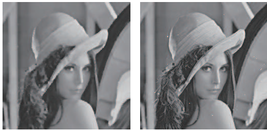
(a) Output image of median filter. (b) Output image of progressive switching median filter.
