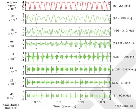
**Fig. 2.** Wavelet decomposition of a vibratory signal corresponding to flaking path defect (depth 157 $\mu$ m) at speed of 1500 rpm with wavelet sym7.
