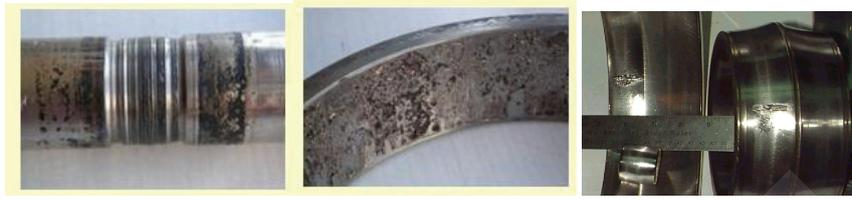
**Fig. 1.** Examples of “Unbalanced Force Defect’s” effect on turning plant’s rotation axis (left) and “Flaking Path Defect” in a bearing device (middle and right).
