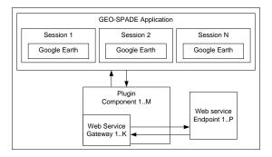
Figure 2: GEO-SPADE architecture.
