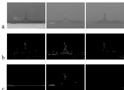
Figure 7: Results comparison on the Liberty Statue dataset: unprocessed image (a); edge extraction results with the proposed algorithm (b); edge extraction results with Canny operator (c).
