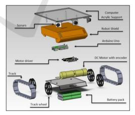
Figure 1: Mechanical structure of the TraxBot.
