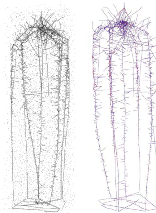
Figure 1: A simulated maize root MRI image at SNR 150 (left) and its true and fitted structure model overlaid, with missing/additional pieces marked in strong red/blue (right).
