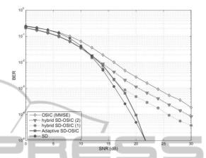
Figure 5: BER performance of the adaptive SD-OSIC system vs. SD, OSIC, and hybrid SD-OSIC schemes.
