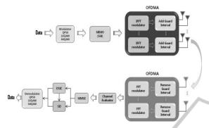
Figure 2: Architecture of the adaptive SD-OSIC system.
