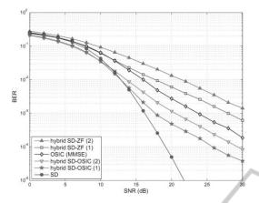
Figure 3: BER performance of hybrid SD-OSIC vs. SD, OSIC, and hybrid SD-ZF.
