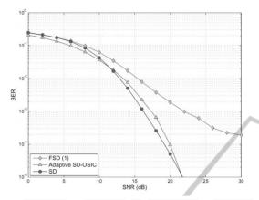
Figure 7: BER performance of the adaptive SD-OSIC system vs. FSD (1)
