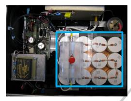
Figure 1: Picture of internal architecture of the nanosecond pulse electric field generator; the pulse forming network is highlighted in blue.
