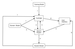
Figure 1: The chess-endgame tutor architecture. The arrows represent the data flow between individual components, and the numbers show the time order of the data interchange in a tutoring session.
