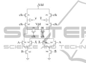
Figure 10: An optimized implementation of an early evaluation free DDPL AND/NAND gate.
