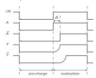
Figure 4: Time diagram of the NOT/BUFFER signals.
