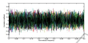
Figure 16: Correlation frequency power analysis on a DDPL S-box without early evaluation (N = 1000).
