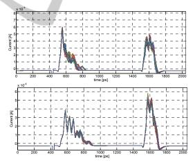
Figure 15: Superimposition of the current traces for the S-Box with (upper) and without (lower) early evaluation.
