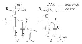
Figure 1: Model of power consumption of an inverter.
