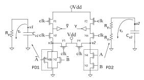
Figure 4: A basic DDPL AND/NAND gate with the equivalent circuits of the evaluation network.
