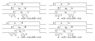
Figure 5: Time diagram of the evaluated signals at the output of a basic DDPL AND/NAND cell for all possible inputs.
