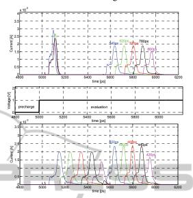
Figure 13: Superimposition of current traces for the multi level logic implemented with basic (upper) and optimized (lower) AND/NAND gates.
