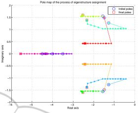
Figure 3: Itineraries of closed-loop poles in optimized eigenstructure assignment based on Hankel program (5).
