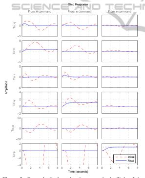
Figure 2: Control of a launcher in atmospheric flight. Initial and final controller obtained respectively by standard and optimized eigenstructure assignment in the case where eigenvectors are not structured. Decoupling is improved.
