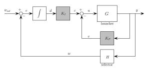
Figure 1: Control architecture with MIMO PI-controller.
