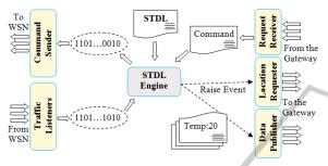
Figure 2: The Components of the Proxy.
