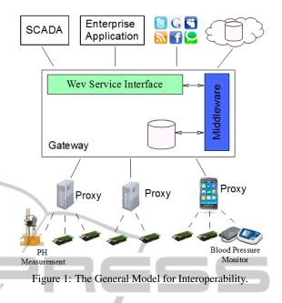
networks. The gateway allows front-end applications to interact with sensor networks, acting as a bridge between the sensor networks and the Internet. Both proxy and gateway may also comprise some other facility services such as authentication and authorization.
