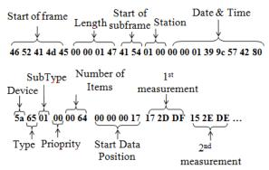
Figure 7: An Example of a Complex Frame Containing a Data Table.
