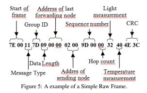
The STDL description of this frame is shown in Fig. 6. In this example, it is assumed that the only information needed is the sending node identification and the light and temperature values. Consequently, the content element of the frame description only comprises three elements: *senderId*, *light* and *temperature*, respectively (see Fig. 6).
