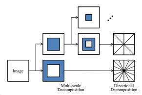
Figure 1: The non-subsampled contourlet transform for the image decomposition.
