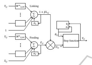
Figure 2: Block diagram of a single neuron of the PCNN.
