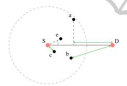
Figure 1: Comparison of geographic algorithms. Node a is chosen by MFR algorithm, node b by Greedy, node c by NFP and node e by Compass.
