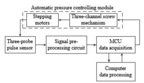
Figure 2: The block diagram of the hardware of threechannel self-pressurized pulse acquisition system.
