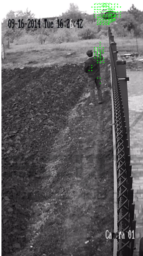
Figure 2: Detected optical flow on the foreground of the image. Only flow vectors with length greater than 1 are shown.
