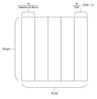
Figure 4: Vertical Slice Method.
