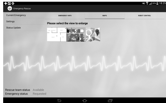
Figure 4: A screenshot of the developed mobile app for the ERTs that shows the availability of three maps, i.e., map for ARTOS location in the home environment, the home environment 3D map, and the Google map to the elderly person home. Clicking on any of them shows in full screen the selected map.
