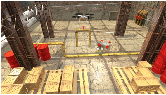
Figure 1: Heterogeneous symbiotic robotic system deployed on a mission to close a valve in a disaster stricken industrial environment.
