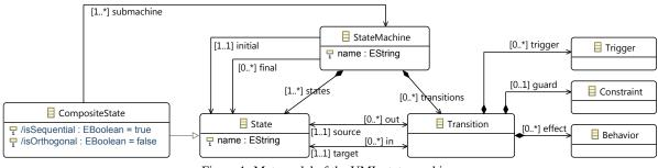
Figure 1: Metamodel of the UML state machine.
