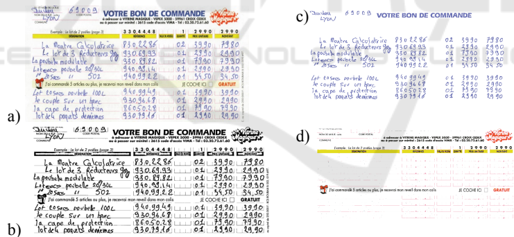
Fig. 7. Color segmentation outperforms the adaptative tresholding (Sauvola) of the lumiance for character segmentation.
