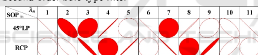
Figure 3: Calculated spectral variations of SOP_{out} 's of four filters with respect to two specific SOP_{in} 's such as 45° LP and RCP.
