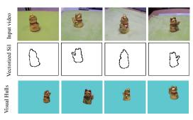
Figure 7: Silhouettes vectorization in eight video streams and Visual Hull rendering based on the silhouettes. The first row shows 4 channel video images(eight in total), the second row is the corresponding vectorized silhouettes. Visual hulls are rendered from different viewpoints based on the silhouettes(the third row).
