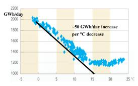
Figure 1: Correlation between temperature and electrical consumption in France – Gradient of daily consumption in France in GWh/day as a function of the average temperature in France (in °C).
