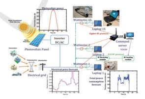
Figure 11: Real time control of 15 laptops charging/discharging for demand response.
