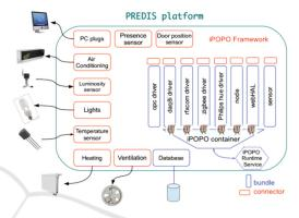
Figure 10: Sensor/actuators interoperability framework.
