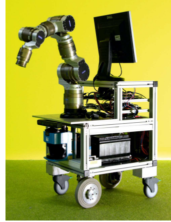
Figure 2: Non-holonomic omnidirectional manipulator with n = 2 actuated wheels. The laser scanner marks the front side.
