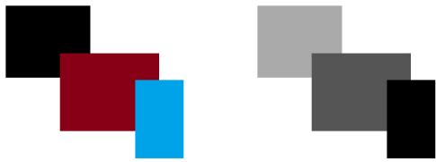
Figure 4: On the left, the original image where the three polygons overlap with each other. On the right, the result after applying the algorithm. The black color corresponds to the value of depth three, thus making the rectangle on the right is ahead of the depth. Furthermore, how strong is gray, the greater the depth value.
