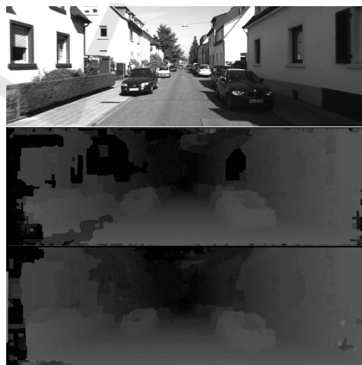
Figure 5: The bottom image is the result of SBM, the second image depicts the disparity map using a sparse census descriptor and the first image represents the left intensity image.
