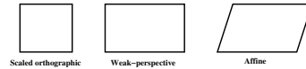
Figure 1: Pixels for different camera models. Scaled orthographic, weak-perspective and affine camera pixels are equivalent to square, rectangle, and parallelogram, respectively.
