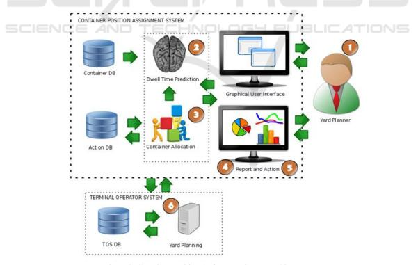
Figure 2: Container Position Assignment System architecture.
