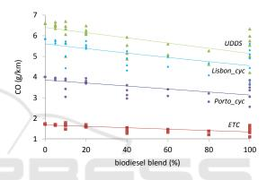
Figure 5: Engine CO emissions function of the biodiesel blend for the four simulated driving cycles.
