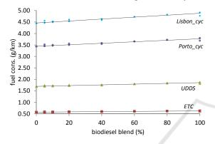
Figure 3: Engine fuel consumption function of the biodiesel blend for the four simulated driving cycles.
