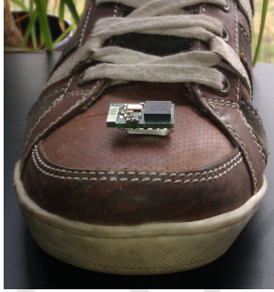
Figure 8: Topview of the micro-IMU V3 which is mounted on a shoe.
