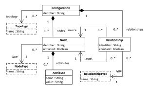
Figure 5: Configuration metamodel - Runtime.
