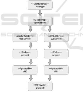
Figure 9: A reconfiguration from our motivating example (SaaS level).
