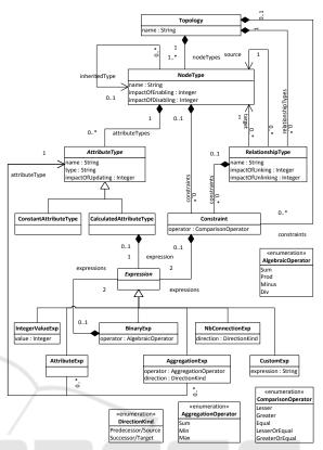
Figure 4: Topology metamodel - Design time.
