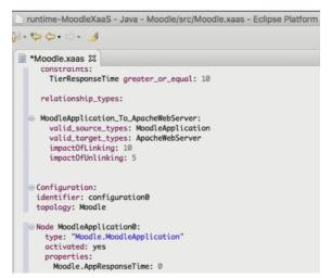
Figure 7: Screenshot of the developed Eclipse-based XaaS modeling environment.
