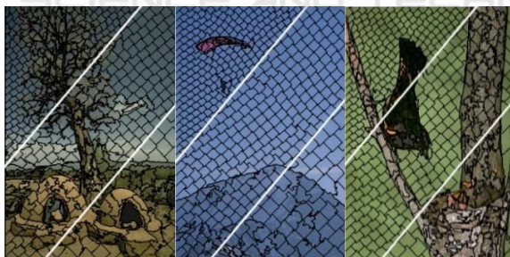
Figure 1: Image segmentation using mDBSCAN algorithm. The number of superpixels are 250, 500 and 1000, respectively.
