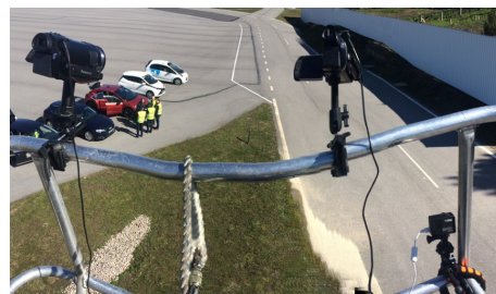
Figure 3: Panorama snapshot of three out of four cameras from the observers perspective. The calibration technique incorporates known distances between cameras. The distance between the top cameras is 77cm, the distance between the top left and the bottom right camera is 127cm. The basket size is 120 \times 60 cm, its height is 120cm.
