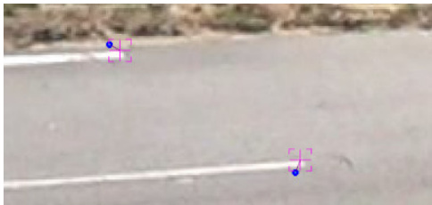
Figure 5: Example for the reprojection error (here \approx 12 px for both reprojected points shown in blue): The image depicts a small part of the calibration image of \text{SET}^{(3)} , \text{CAM}_3 .
